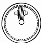
916. WORM-GEAR PINION to drive an internal spur-gear wheel.
