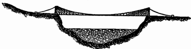
1509. SUSPENSION BRIDGE.—Niagara upper bridge, "Roeb- ling" system. Twelve hundred and fifty feet between piers.
