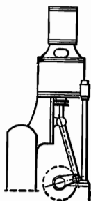
231. TANDEM COMPOUND VERTICAL ENGINE, with continuous piston rod.
