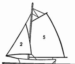
767. SLOOP.—A mainsail and jib with fore- and back-stays. 2, jib; 5, mainsail.
